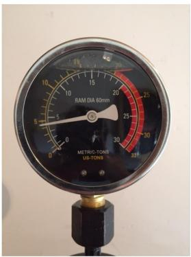
No First crack Collapse at 4.5 tons
