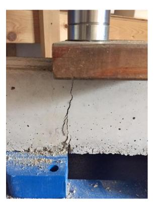
First crack at 1 tons Collapse at 2 tons
